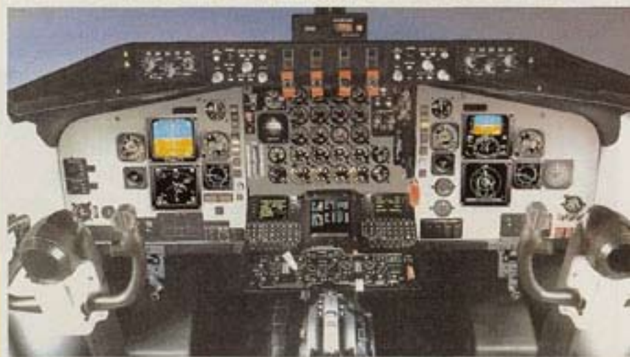
USAF KC-135s have undergone ATM interoperability upgrades, including automatic dependent surveillance and controller pilot data link communications. An earlier program added traffic and terrain warning. Old (top) and new cockpits are shown above.
